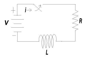
When the switch is closed on the above circuit, the instantaneous current, as a function of the short circuit current is given by:
