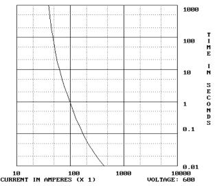
Figure 2 above is the average melting time current curve for a 30A, 600 VAC fuse that is also UL listed for 500 VDC to UL 198L standards. The time constant, "tc" of the DC circuit where the fuse is applied must be known before this curve can be converted for DC use. The procedure for converting a time current curve is presented as follows:
