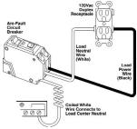
Diagram A. 1-pole 120Vac 2-wire branch circuit
