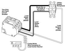
Diagram D. 2-pole 240Vac load application derived from 120/240Vac
